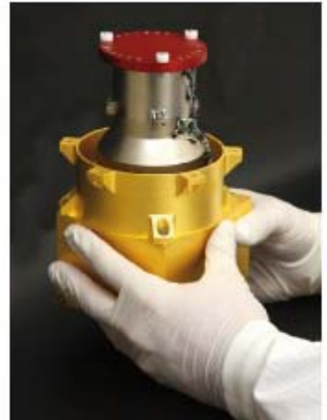
Kiel University is responsible for the heart of the Radiation Assessment Detector (RAD), the actual detector (RSH – Rad Sensor Head) that measures the cosmic radiation.
